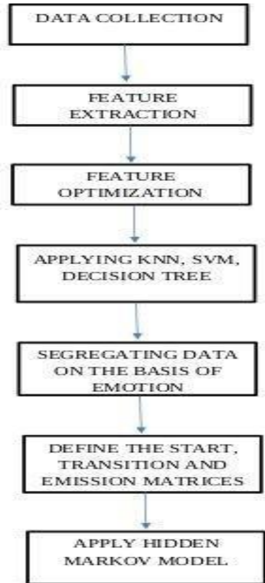
Fig. 1. Approach for Emotion Detection using MFCC and HMM
