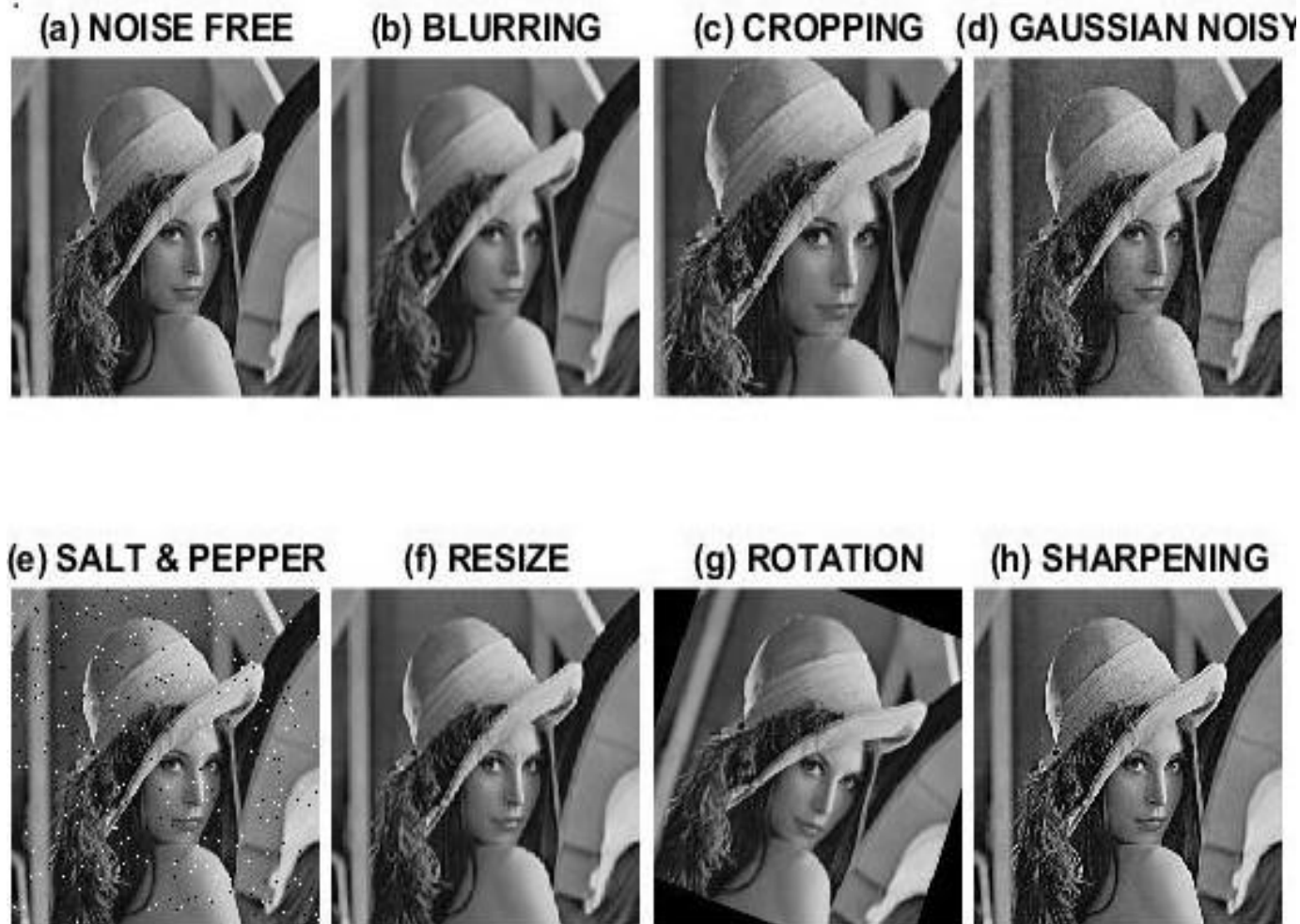
Fig. 1. Effect over Lena image (a) without any attack (b) with blurring (c) with cropping (d) with addition of Gaussian noise (e) addition of Salt & Pepper noise (f) with resizing effect (g) with rotation attack (h) with sharpening attack.
