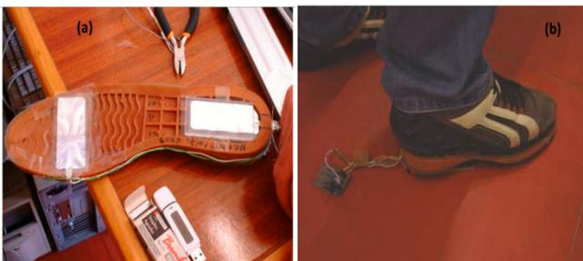
**Fig.5. Photograph showing (a) the position of the electroactive films on the shoe sole (b) the harvester integrated into the shoe along with electronic circuit**
